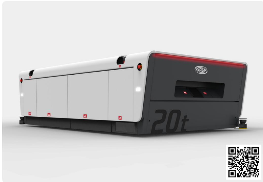
Jaso's steerable self-driving carts are suitable for moving all types of load at ground level, both indoors and outdoors.
